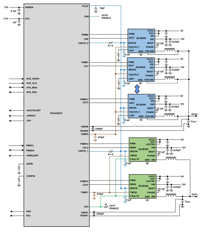
Figure 1. 14+2 Smart Power Stage
